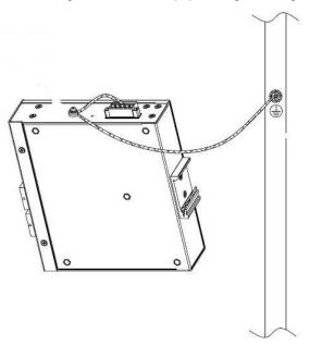
Figure 3-4 track Ground completion schematic
