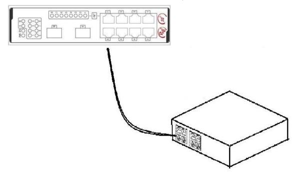
Figure 3-7 Connecting Base-T ports and other Ethernet terminal
