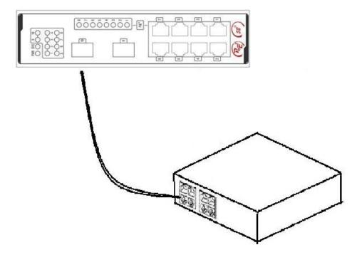
Figure 3-5 Connecting the SFP ports and other Ethernet terminals
