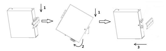
Figure 3-2 track installation diagram
