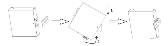
Figure 3-1 track installation diagram
