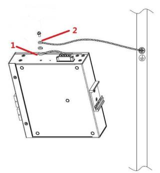
Figure 3-3 track Equipment grounding
